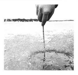
Tape measure: Use a tape measure to find ice's true thickness. Put the tape measure into the hole and hook the bottom edge of ice before taking measurement. You can also use an ice fisherman's ice skimmer with inch markings on the handle in place of the tape measure. Don't judge ice thickness by how easily a chisel or drill breaks the surface. It happens so quickly that it's easy to overestimate the thickness.
